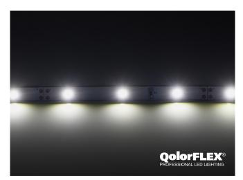
**QolorFLEX LED Tape, Natural White, 12V Indoor** (P/N 3528-12-NW-30-5-20-1) is an economically priced interior grade LED tape with a medium/low output (165 lumens/metre) brightness. Intended for applications where high light output is not required, the natural white colour (4100°K) is ideal for use where good colour rendition is needed. Each LED tape comes with wiring leads on both ends and durable 3M adhesive backing. It is available in full five metre reels and sample strips.
